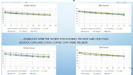
We added 150ml of hot water into each cup and recorded the temperature using a thermometer. We then recorded the temperature every 2 minutes for 16 minutes.
